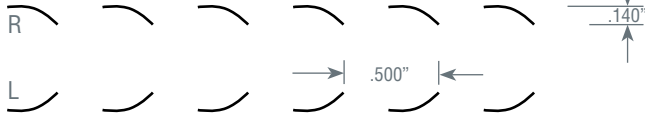
4D – 1/2" Pitch (12.7mm) 3/16" Gap (4.75mm) right hand and left hand zipper rule
