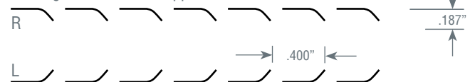
4T – .400" Pitch (10.10mm) .250" x .150" (6.35mm x 3.81mm) right and left hand zipper rule
